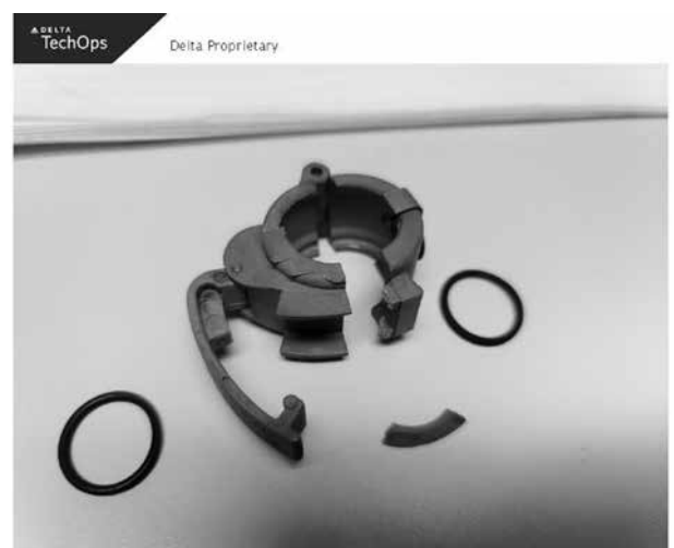
The clamp (red) which when closed secured a pipe join. [Photo courtesy of Delta TechOps, reproduced from the Official Report]
