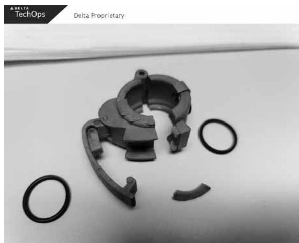
圖3: 夾具扣(紅色) 扣緊時可固定管線接合處 (Source: Delta TechOps, reproduced from the Official Report)
