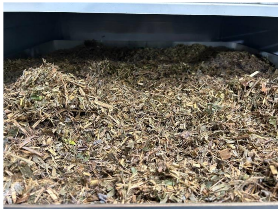
Crushed Pennisetum to be burned into biochar.
